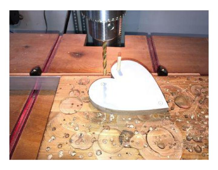
Stacj the top and bottom to drill the holes. The holes in the top and bottom are 1/4" diameter. We will use 1/4" wooden dowel for the pivot shafts.
