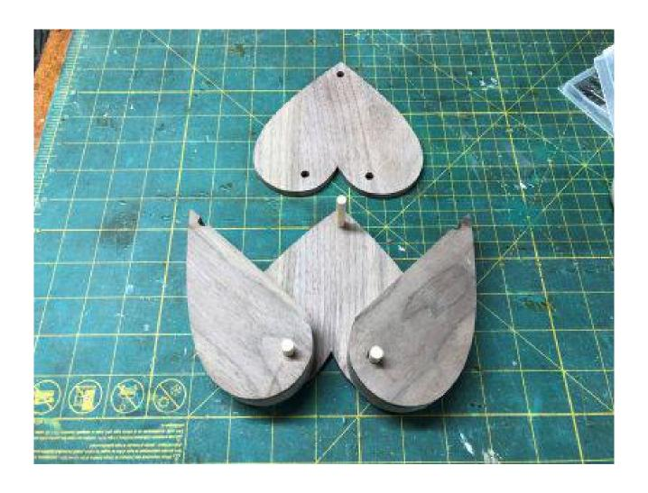
Cut the dowels long. Insert the dowels in the top and glue in place. Slide the drawers on the wooden dowels being carefull dot to get glue on the drawers.
