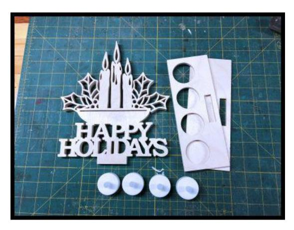
If you cut the slot and tab joint tight enough you can Eliminate the glue so you can pack it flat. I did end up gluing the base together but left the fretwork free.
