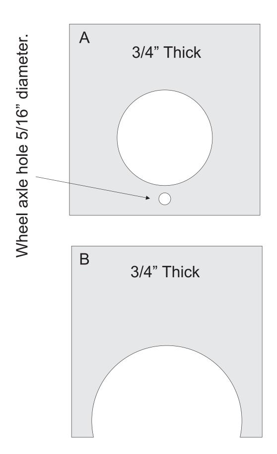
Stack pieces A and C to drill the 5/16" hole for the axle.
