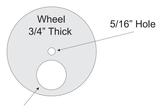
Taper the edges to prevent the gumballs from Binding
