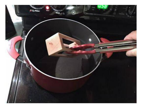
Now for the magic. Heat 3 inches of water to a boil. Remove the pan from the burner and submerge the wood blank in the water for 15 minutes.
