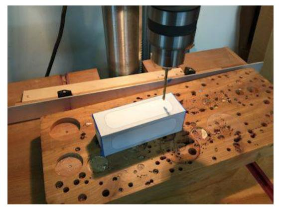
Drill the entry holes on both sides of the pattern.
