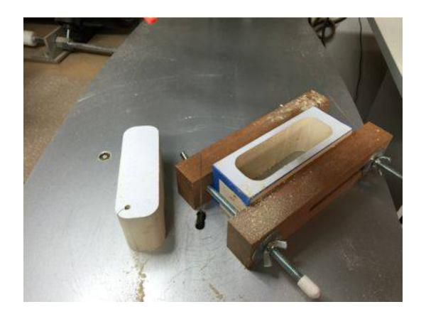
After you finish the first cut flip the blank. Keep the waste piece in the blank and complete the second cut.
