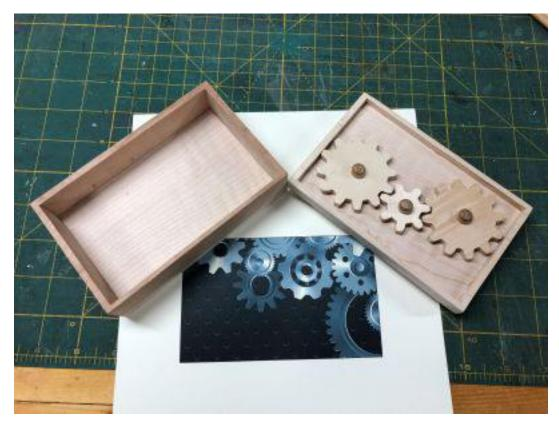
Print the optional graphic of photo paper. Glue it in to the bottom of the box. When I finished the box with spray lacquer I sprayed over the graphic also.
