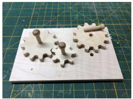
I used axle pegs for the gear shafts. I used pegs with a 7/32" shaft diameter but any pegs will work.
