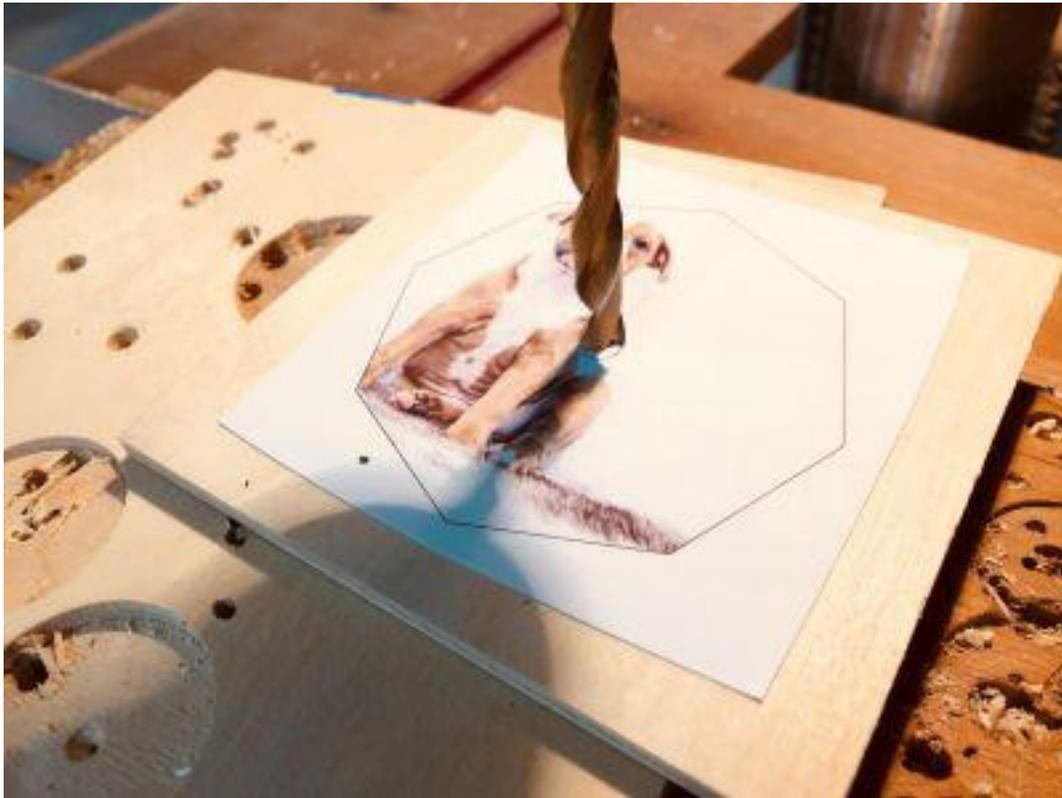
Use a backer board. Line up the drill bit with the center punch. Place a front board. Drill the hole.
