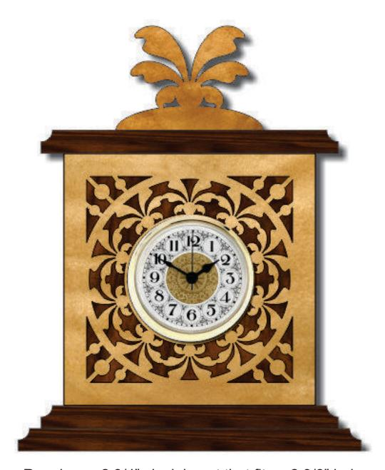
Requires a 2 3/4" clock insert that fits a 2 3/8" hole It is recommended to cut the hole with a 2 3/8" forstner bit for the best fit. If you use your scroll saw cut just inside the line and sand to a snug fit of the clock insert.
