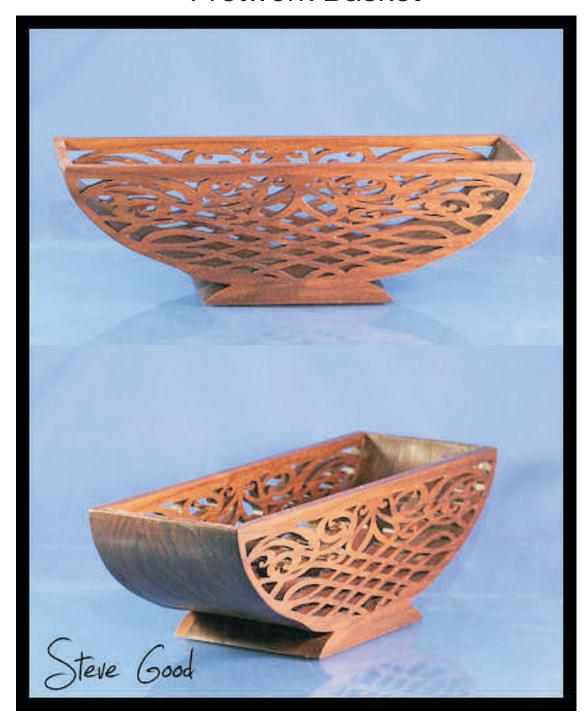
Stack cut the two side pieces to reduce the time it takes to cut the project. After all the pieces are cut glue the centerpieces together and let them dry. Sand the center assembly smooth before you glue on the sides. It makes sanding much easier. Glue on the sides and sand them flush to the center assembly.
