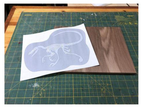
This pattern comes in two sizes. The smaller one will be more difficult to cut because of the bevel. You will have to be very precise when you cut the bevel on the small pattern.
