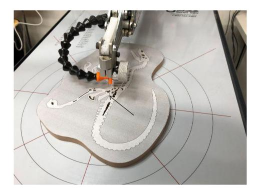
To prepare for the bevel cut drill a in a spot that will not be obvious. Carefully cut around the fossil.
