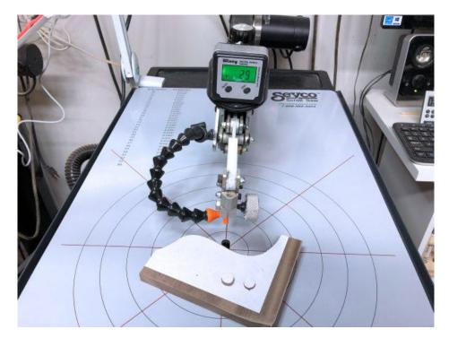
Now it's time to make the test cut for the bevel. I used a #1 blade and 1/2" thick wood. My angle came out to ~3 degrees. Yours will vary depending on your blade and thickness of material.
