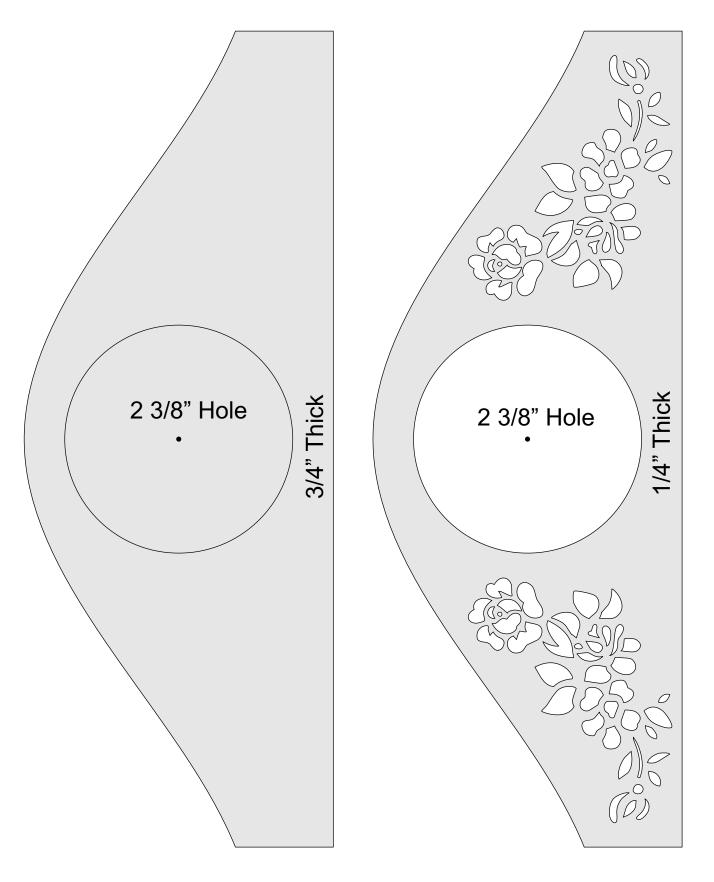
If you have a 2 3/8" forstner bit use it for the clock insert hole. If not just use the scroll saw and slightly undersize the hole. You can sand the hole for a good insert fit.
