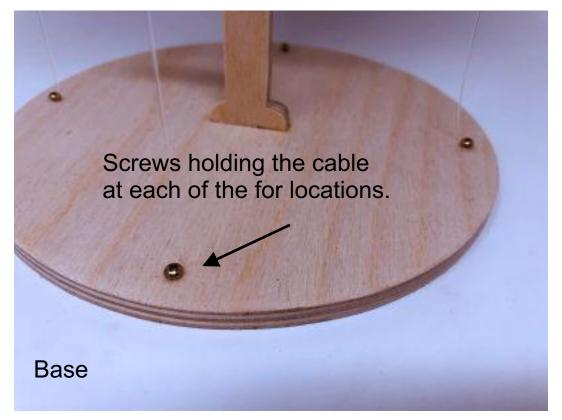
Cut the fishing line extra long. Screw the line to the base. Glue the center bracket into the base and let the glue dry.
