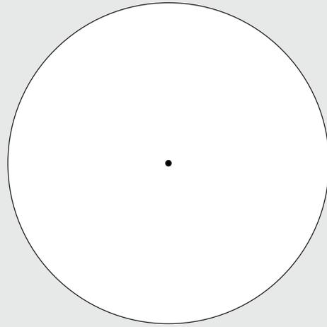
You can cut the hole with the scroll saw or a 2 3/8" forstner bit.
