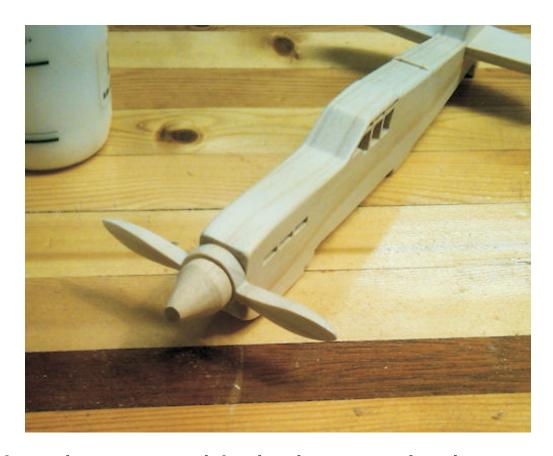
Glue the assembled wings to the bottom of the fuselage.
