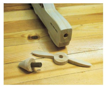
Glue a piece of dowel into the nose cone.
