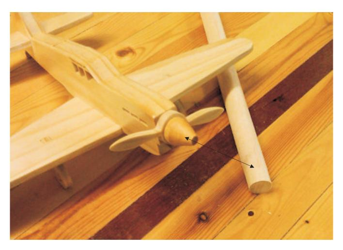
Taper the cone before you cut it off the dowel. It's hard to hold after you cut it off.
