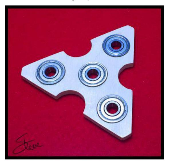
Use two part epoxy to set the bearings in place. The three outer bearings are just there for weight and can be replaced with other weighted objects. If your hands are small shorten the three tips.
