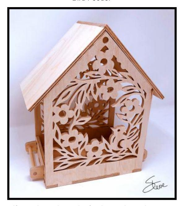
If you plan to hang the feeder outdoors then use exterior wood glue on all the joints.
