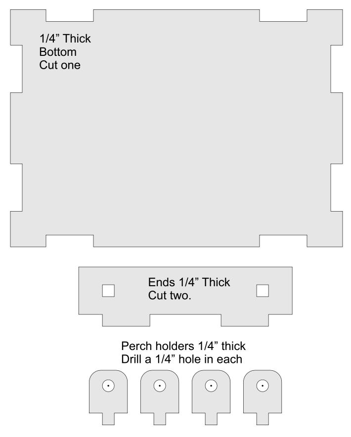
Cut two 1/4" diameter wooden dowels to a length of 3.5"
