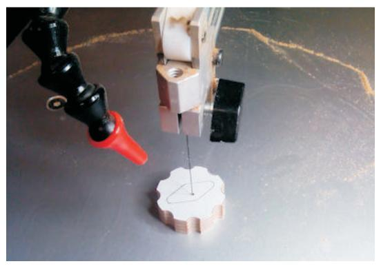
Carefully cut out the interior hole. Because you traced the plastic at the smallest potin of the taper you will want to cut on the outside of the line. As you push the clamp into the hole the taper should make for a nice tight fit.
