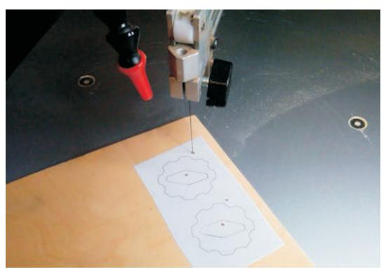
Drill your entry holes and prepare to cut out the knobs.
