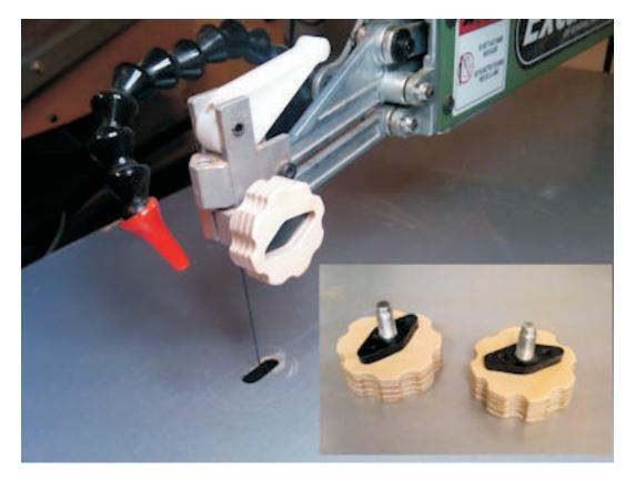
The T style knobs that come with the Excalubur scroll saws can be uncomfortable. Why not use the scroll saw to make a set of knurled knobs for better comfort. The picture above shows the top knob in place. These knobs are simply press fit over the plastic T so they can be removed easily and replaced if they break.
