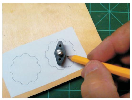
With a very sharp pencil trace the outline of the blade clamp. Note the orientation of the clamp on the knob. Make sure it is centered and pointed to a high spot on the knob.
