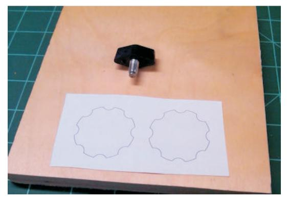
Apply the pattern to the plywood with spray adhesive.
