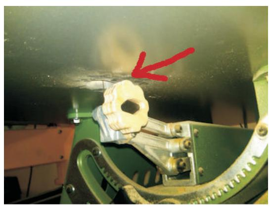
This is a picture of the knob installed on the bottom blade clamp. The picture above shows the lower arm in it's highest position. In this position it's still a little difficult to turn the knob. I suggest you push the arm down so you have more clearance like the picture below. Now you have plenty of room to grip and turn the knob.
