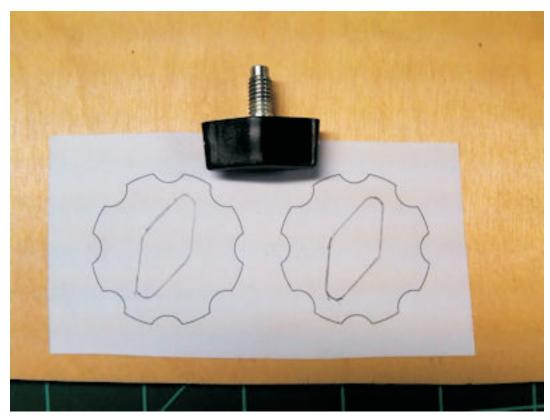
Note the taper of the plastic on the blade clamp. Because of this taper the clamp will fit very snug if you cut just to the outside of the outline you drew. Experiment for the fit you like.
