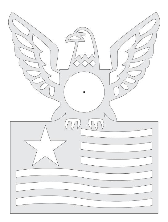
Requires a 1 7/16" mini clock insert. Use a 1 3/8" Forstner bit to drill the hole.
