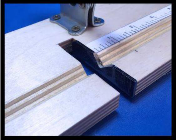
Steel insert cut from a flat wrench. I used a Dremel tool to cut the insert to length and make the V-notch.
