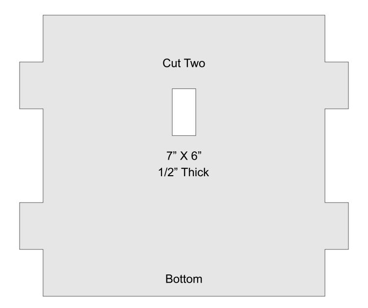
Bottom of the Box 1/4" Thick Measure the box and cut this part to fit.
