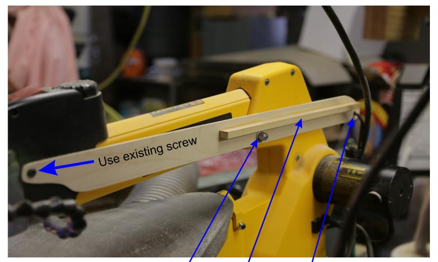
Replace original bolt with 1/4 x 3" bolt, flat washer and hex nut. Do not tighten, must be loose to allow arm to piviot
