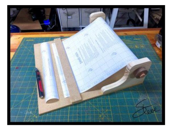
Attach the roll end blocks to the base board with glue and flat head nails.
