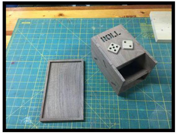
Glue the bottom lip to the bottom. Clamp and allow the glue to dry. Sand to desired finish. Apply desired finish Install felt in bottom.
