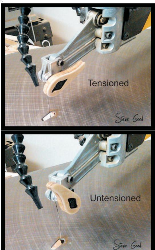
Cut the opening for a tight fit to the existing thumbscrew. I used 3/8" Baltic birch Plywood for strength. Sand all edges smooth for comfort.
