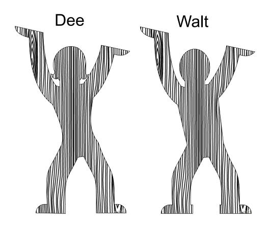
Run the grain as shown for most strength.
