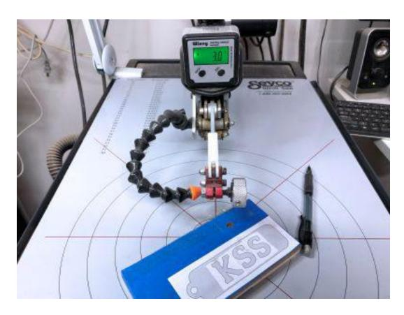
I like to cut in a counterclockwise direction so I moved the tile of the blade to the left. I adjusted the angle to 3 degrees. This is 1 degree larger than the last test cut.
