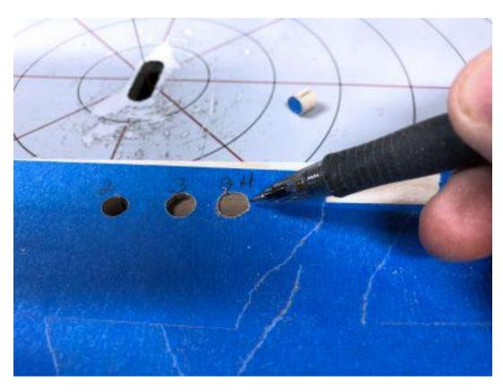
Here is the back side of the board with the blade at 2.4 degrees. Note that the walnut is just slightly below the surface. This is exactly what we want.
