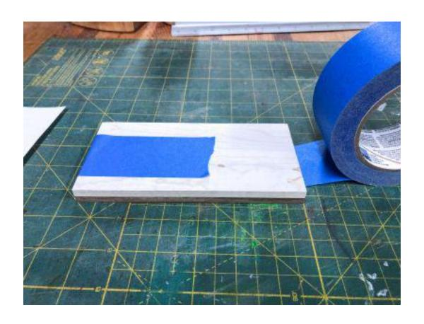
Wrap the two pieces of wood with the blue painters tape. We will be cutting both at the same time.
