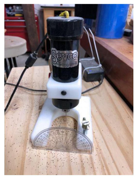
It is not absolutely necessary but drilling the interior holes at the same angle the blade is tilted can sometimes make the entry hole less obvious in the final project.
