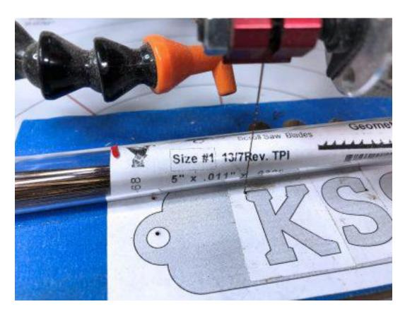
I am also going to use a small scroll saw blade. I'm using a #1 blade. This is again not absolutely necessary but it make the turn of the cut much easier and generally gives to sharper letters in the end.
