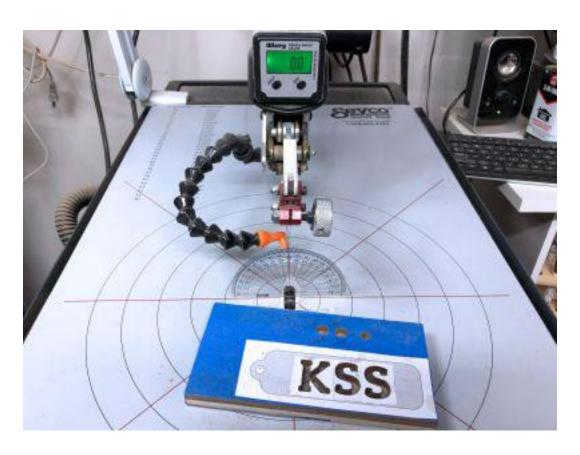
After all three letters have been cut we need to set the blade back to 90 degrees to cut out the key fob exterior.
