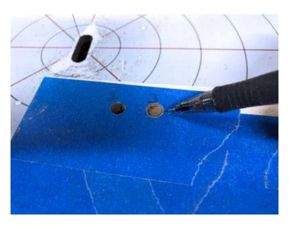
Here is the back side of the second test cut at 3 degrees. Note that the walnut does not come out the bottom.
