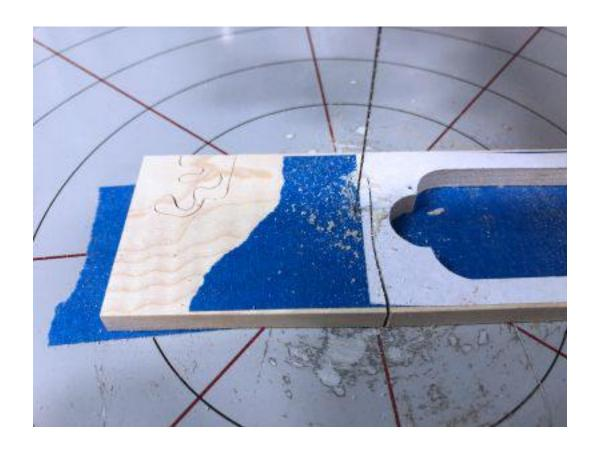
We are going to make out own wood putty to hide the drill entry holes.
