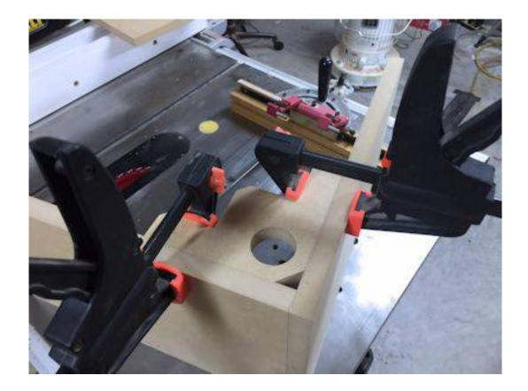
Use quick release bar clamps as shown above or spring clamps below. The bar clamps provide more secure clamping.
