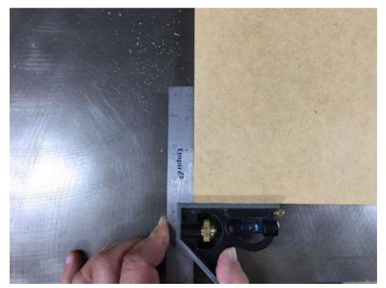
Make sure the edges that will go against the box are a perfect 90 degree angle. Best to use the factory cut edge or cut with a well adjusted table saw. You can use the scroll saw to cut all other edges.
