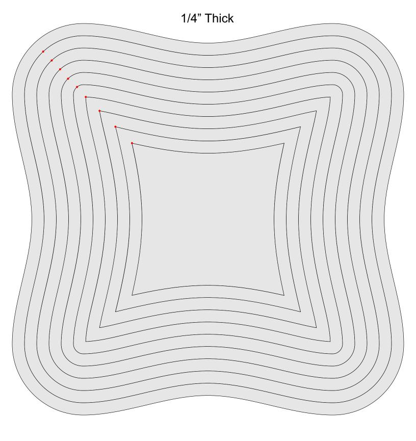
Use the smallest drill bit you have to minimize the hole. After the rings are cut you can sand the blemishes away.
