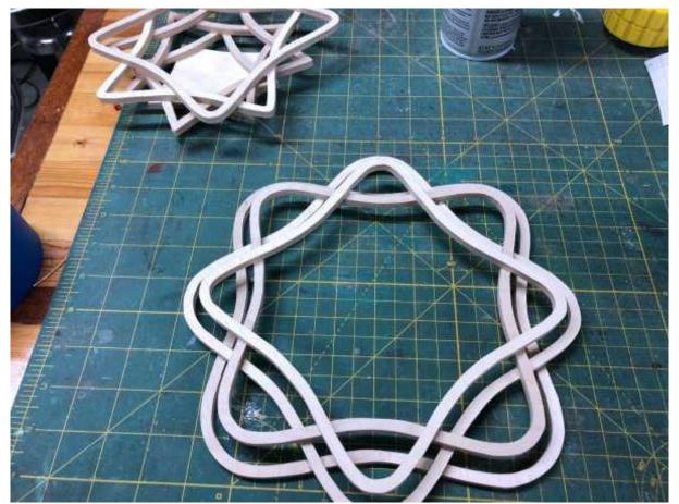
I assemble from the top up. I lat the first ring down. Place the next ring on top and mark with a pencil for the glue. Continue until the stacks are complete.
