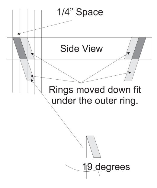
I add 1 degree to the actual angle when I cut the pattern. This compensates for the thickness of the blade.
