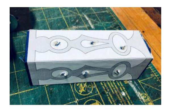
Drill the interior holes on each side.
