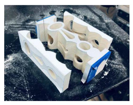
You have just cut off the side two pattern. We have to replace it. Carefully tape all the pieces back together leaving the side two pattern visible.
