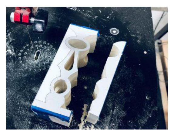
Remove the blank from the clamp and cut the exterior on side one right. Then cut side one left.
