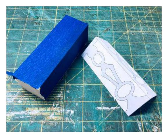
Wrap the pattern around two sides of the blank. I used the blue painters tape to make the pattern easier to remove
