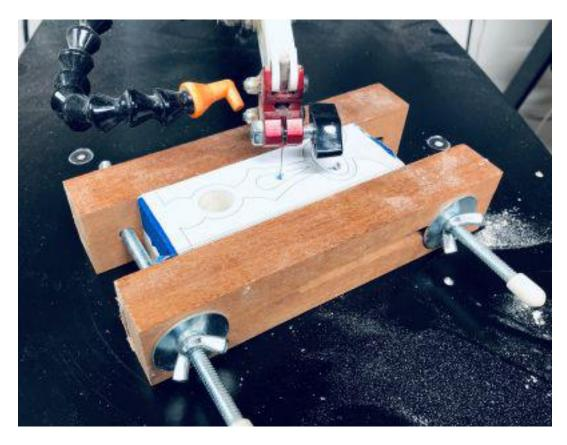
Cut the interior cuts on side one. Flip the wood and cut the interior cuts on side two.
