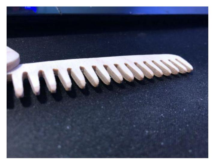
I kept the teeth of the comb large to help prevent breaking. The comb works best if you sand the teeth to a blunt point.
