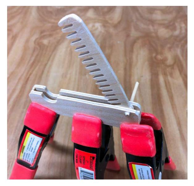
Clamp the body together and before the glue dries insert the 1/8" dowel through the body and comb. Use a small amount of glue at one end of the dowel to hold it in place.
