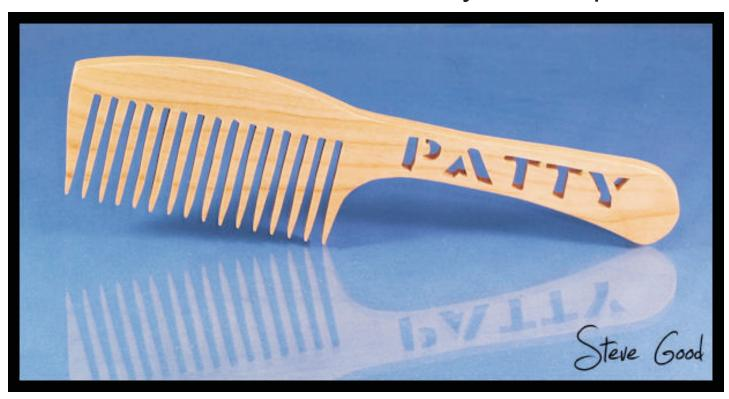
The direction of the grain on this comb is not the best for strength. Try to cut the blank so the grain runs in the direction of the teeth.
