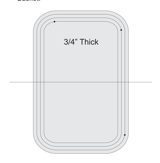
Drill 1/4" Hole for pivot dowel only in the outer ring.
