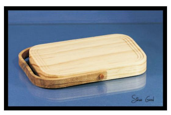
Set your scroll saw table to 3 degrees. Test cut on scrap to see that the basket will collapse properly. Set the table back to 90 degrees for the outside cut of the Basket.
