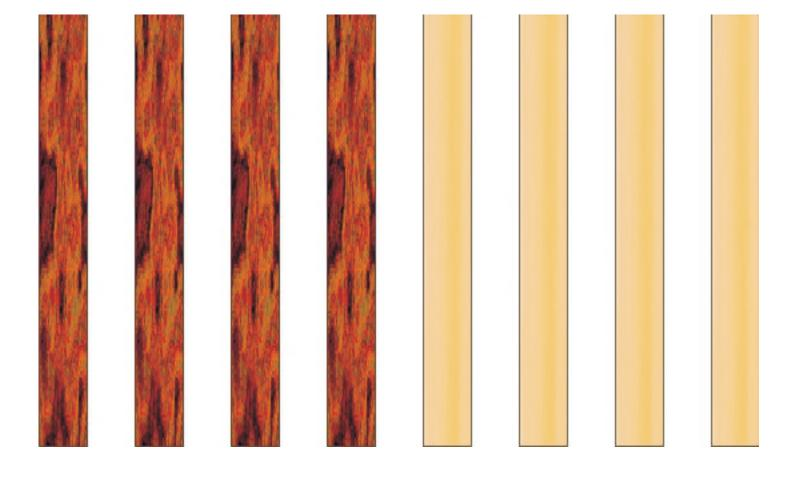
Glue the boards up alternating dark and light. Glue and clamp until the glue dries.
