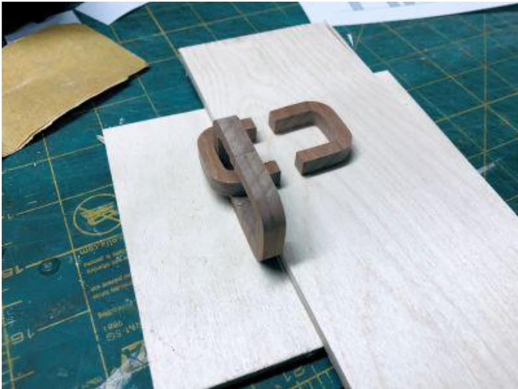
When I do the glue up I use two board the same thickness of the links to make a stair step. This make it easier to do the glue up. I only clamp with finger pressure. I hold each link for a couple of minutes. Then I move to the next link.
