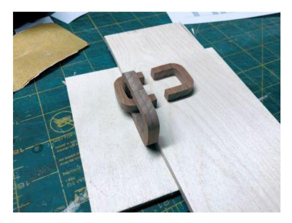
When I do the glue up I use two board the same thickness of the links to make a stair step. This make it easier to do the glue up. I only clamp with finger pressure. I hold each link for a couple of minutes. Then I move to the next link.
