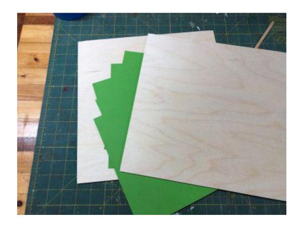
We are going to cut several cards at the same time. Sandwich all the sheets of card stock between two sheets if 1/8" Baltic birch plywood.
