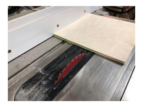
The final stack needs to be 9.5" X 7". I am running the stack through the table saw to get it down to size.
