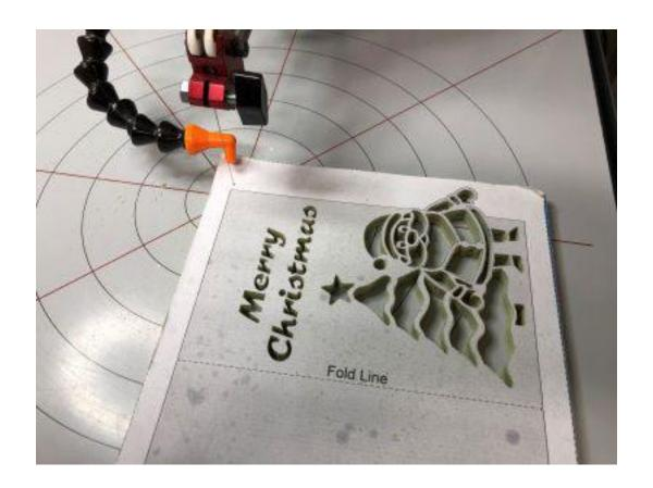
After you finish all the interior cuts it's time to cut the perimeter. Not the small notches ate the fold line. Use the blade to make a small cut at the notches. This cut will make it easier to find the fold line.
