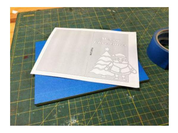
Wrap the stack in blue painters tape. Use spray adhesive to glue the pattern to the stack.
