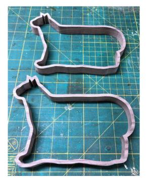
To get the thickness of the box you need 1.5" thick wood. If you do not have wood that thick then glue up two 3/4" thick boards.
