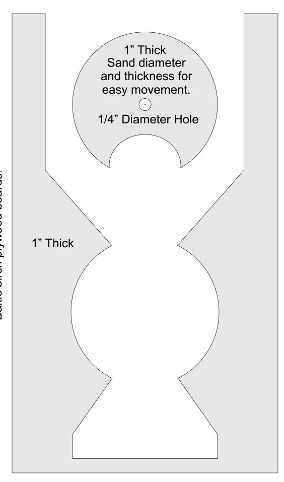
I glued up two 1/2" thick Baltic birch plywood boards.
