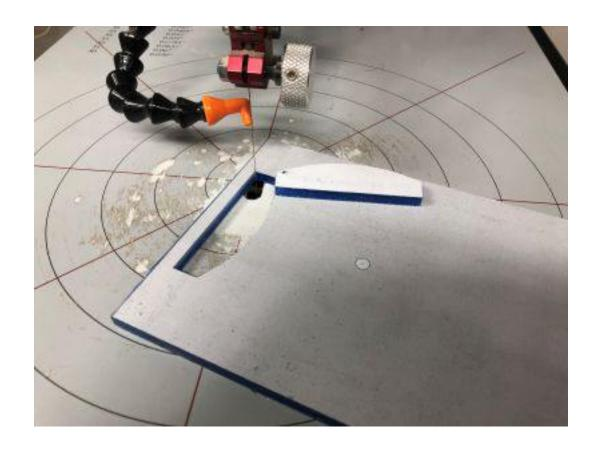
Cast acrylic is the easiest to cut but with care you can cut most acrylic sheets. Cut the sheet to size and carefully drill the hole accurately.
