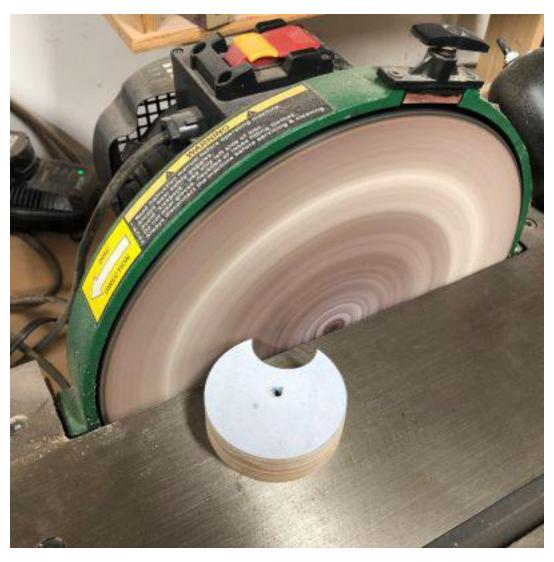
Sand the diameter and thickness of the dial for smooth operation. I sanded of about 1/16" thickness.
