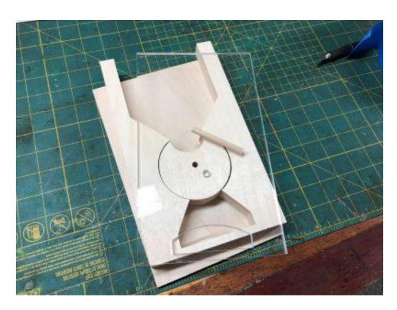
The most critical step is to get the holes lined up so the dial does not bind. Use clamps to hold the pieces together for gluing on the back and drilling the screw holes for the acrylic sheet. Test and re-test as you assemble the pieces.
