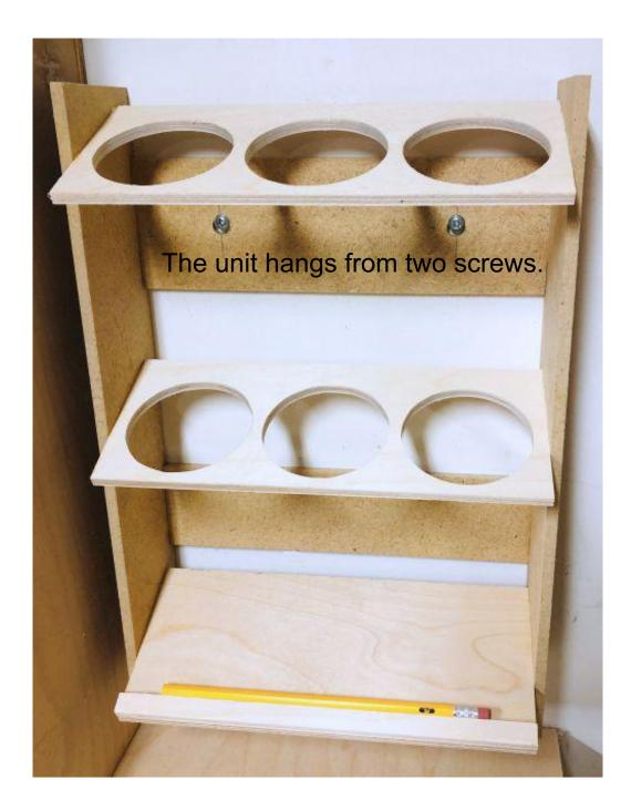
Note that the cans sit on top of the can below. I did it this way to keep the unit as shallow as possible. If you want to use the bottom can you need to slightly lift the can above it.
