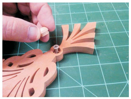
Countersink the screw and use a button or plug to hide the head.
