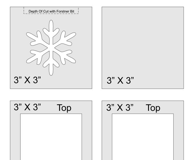
Note that the top of the center pieces is a little thicker. This helps prevent the candle recess from breaking through.
