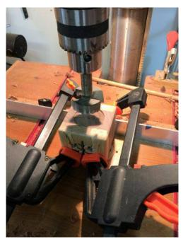
Use a forstner bit in your drill press. For the top use a 2.25 diameter bit. For the bottom use a 1.5 inch diameter bit or one that fits you teal light.
