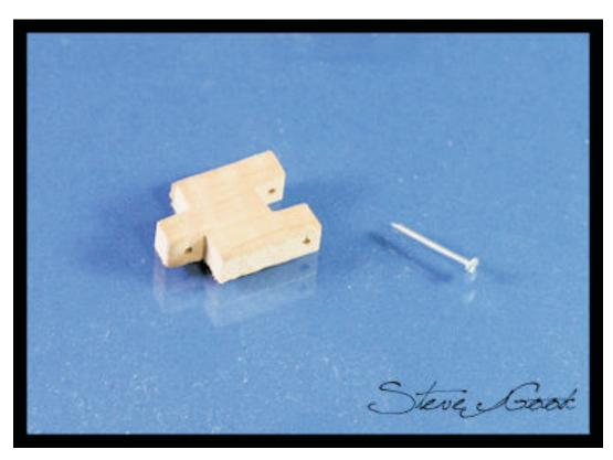
Link with rounded ends. Brad with head cut off.
