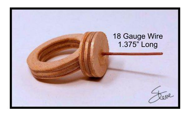
This small tool can be worn on your off hand pointer finger. When you are bottom feeding a scroll saw blade on a large board, you can poke the wire down through the board from the top and line up the blade with the wire.
