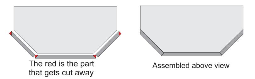
Cut 7 lengths of 1" PVC pipe at 5 3/8 in length Then, cut a 45\* angle on one end of each pipe
