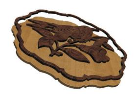
Stack cut the outside of two contrasting 1/4 inch thick boards. This gives an exact fit for the frame. Separate the two boards and cut the interior of the frame. Glue the bird and frame to the bottom plate.
