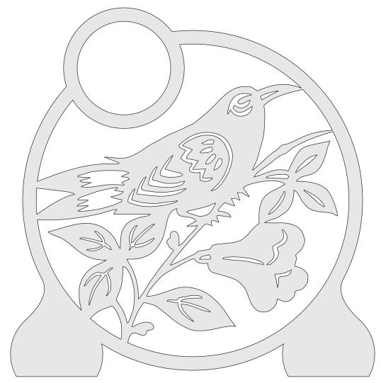
Requires a 1 7/16" mini clock insert. Use a 1 3/8" forstner bit for the insert hole.
