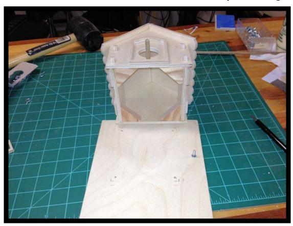
Glue the cleats into the bottom of the colpleted bird house. Pre-drill and counter sink the holes in the base and cleats.
