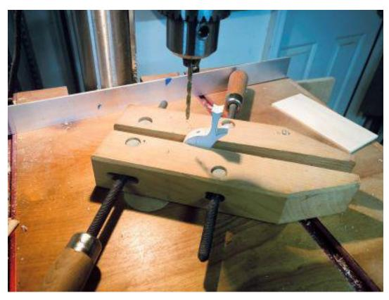
You want the holes in the bottom of the birds to be aligned with the dotted lines on the pattern. If you use a hand drill just be very careful. A drill press and clamp are preferable.
