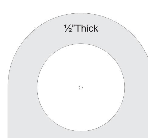
Cut out for a 3 ½" clock insert. Use a hole cutter on a drill press for most accurate cut. Can be cut on the scroll saw also.
