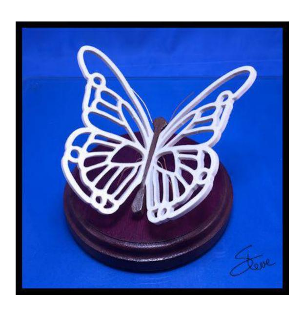
I am using 1/8" thick poplar for the wings and 1/4" thick walnut for the body. I am only going to use one of the wing patterns and stack cut two wings at once.
