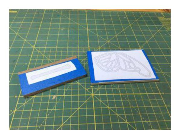
All the interior holes have been drilled and the stacked wings are ready to cut. Cut all the interior holes first.
