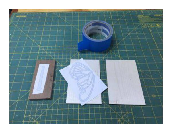
I'm am preparing for the stack cut by taping both 1/8" thick boards together. You don't have to stack cut the wings but it's faster and easier to cut.
