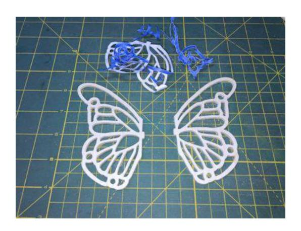
Tilt the scroll saw to 25 degrees. Cut the bevel along both the top left side and the top right side. This bevel is where we will glue the wings.
